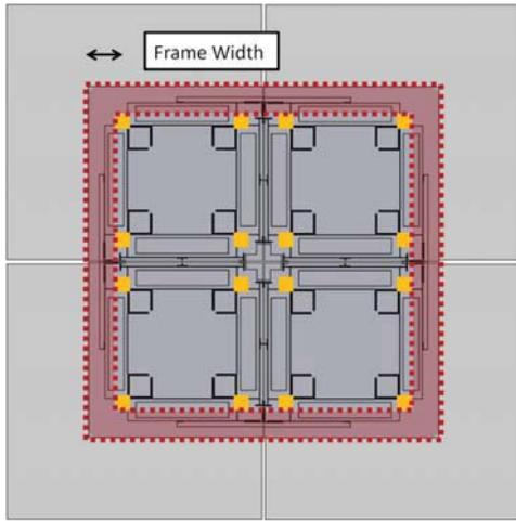
Fig. 8. Diagram of the frame-type die attachment geometry.
